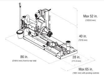
The TCX635 is designed to service truck-type tires with angled bead seats. Passenger car and light-truck tires cannot be serviced on this changer even if they are in the listed clamping range.
