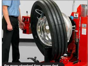
For many standard tires, super-fast double bead mounting is possible.
