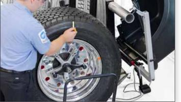
When combining ForceMatch<sup>®</sup> wheel balancer (left) with a heavy-duty tire changer (right), their match-mounting capability achieves the smoothest possible ride.
