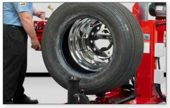
Quickly slide the carriage and spin the tire, rolling both beads off of the rim. It's that easy.
