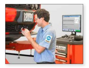
An increasing number of vehicles include advanced driver assistance systems (ADAS). In addition to a mechanical alignment, manufacturer's specifications often require a Safety System Alignment\* on many vehicles equipped with ADAS Systems.
