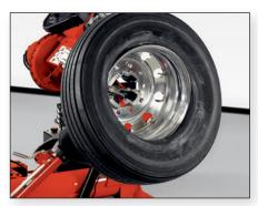
✓ Bead loosening and demounting can be as easy as rolling the tire off of the rim in a single step
