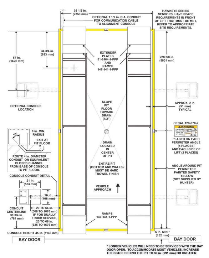
Dimensions shown are for end result. Tile thickness (if applicable) must be considered before pouring concrete. Positioning of control console is limited to a maximum space between console and rack of 5 1/2 feet (1676 mm) at the approach ramp end and 16 feet (4877 mm) at the turnplate end.
