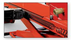
Convenient air source for tools at front and rear
