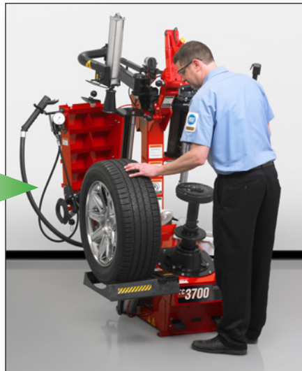
... activate the automated lifting device by pressing the lift foot pedal.
