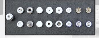
The PR-5 self-piercing rivets join two or more pieces of material with the use of extreme pressure and precision machined punch and die sets. The punches are magnetic to hold the rivets in place, making operation quick and easy. The dies complete the process and prevent the rivet from punching through the last layer of material. This allows you to join different materials such as: aluminum, steel, plastic and more.
