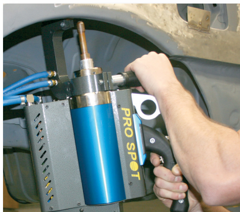
Welding with the Wheel House Arm makes it possible to weld in the most difficult areas.
