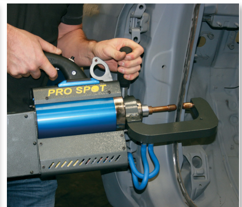
Spot welding of quarter panel using C-Arm
