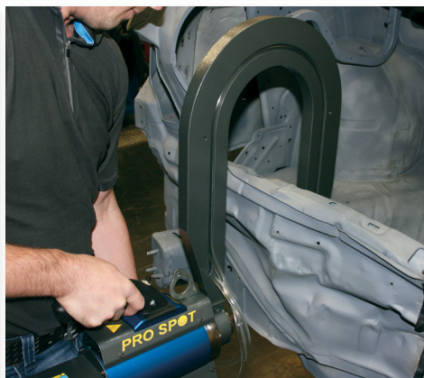
For deeper needs use the Pro Spot extension U-Arms (508mm - 600mm). They are self aligning and quick to install.
